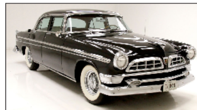
Former U. S. President, Harry Truman's 1955 Chrysler New Yorker sedan. It is fully equipped with a 331 cid HEMI V8, two-speed Powerflite transmission and factory air-conditioning. Mr. Truman purchased this car when he and 'Bess' left Washington, D.C. to return home to Independence, Missouri. --Photo courtesy of Classic Auto Mall
